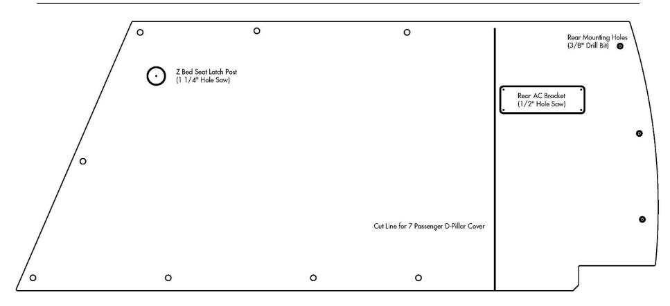
NOTE: If you have an '89-'91 Seven Passenger Van with 3 Point seatbelts in the rear, you will need to cut a hole for the belt to pass through. Make sure to sand the ABS smooth where the belt runs through to avoid belt wear.
