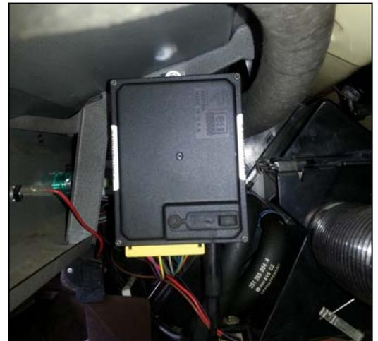
*Note: If for some reason neither of these locations is available to mount the cruise module, another location may be selected by the installer. If selecting a different location, the cruise module **MUST** be mounted so that the dip switches are easily accessible and the cable **MUST** be able to have a nice smooth route to the accelerator linkage.*
