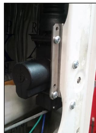
*Note: The brackets include high and low mounting hole locations for the power door lock actuator. Choose the location that clears your door latch bar appropriately.*
